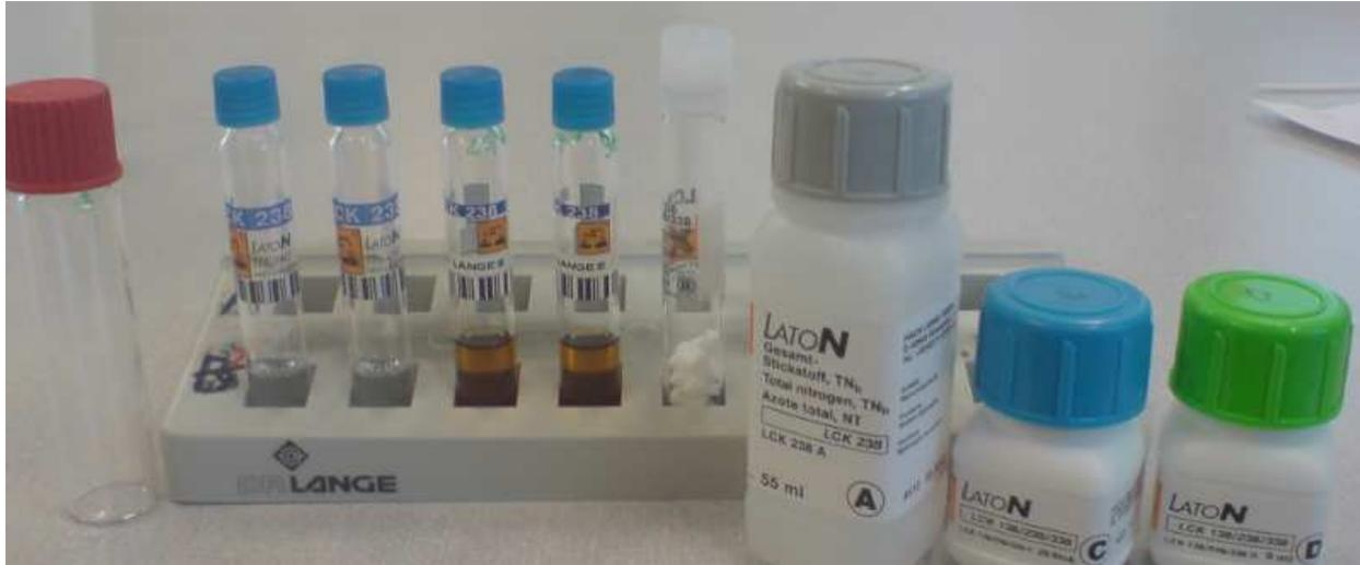
**Figure 9:** Cuvettes and reagents for total Nitrogen test
