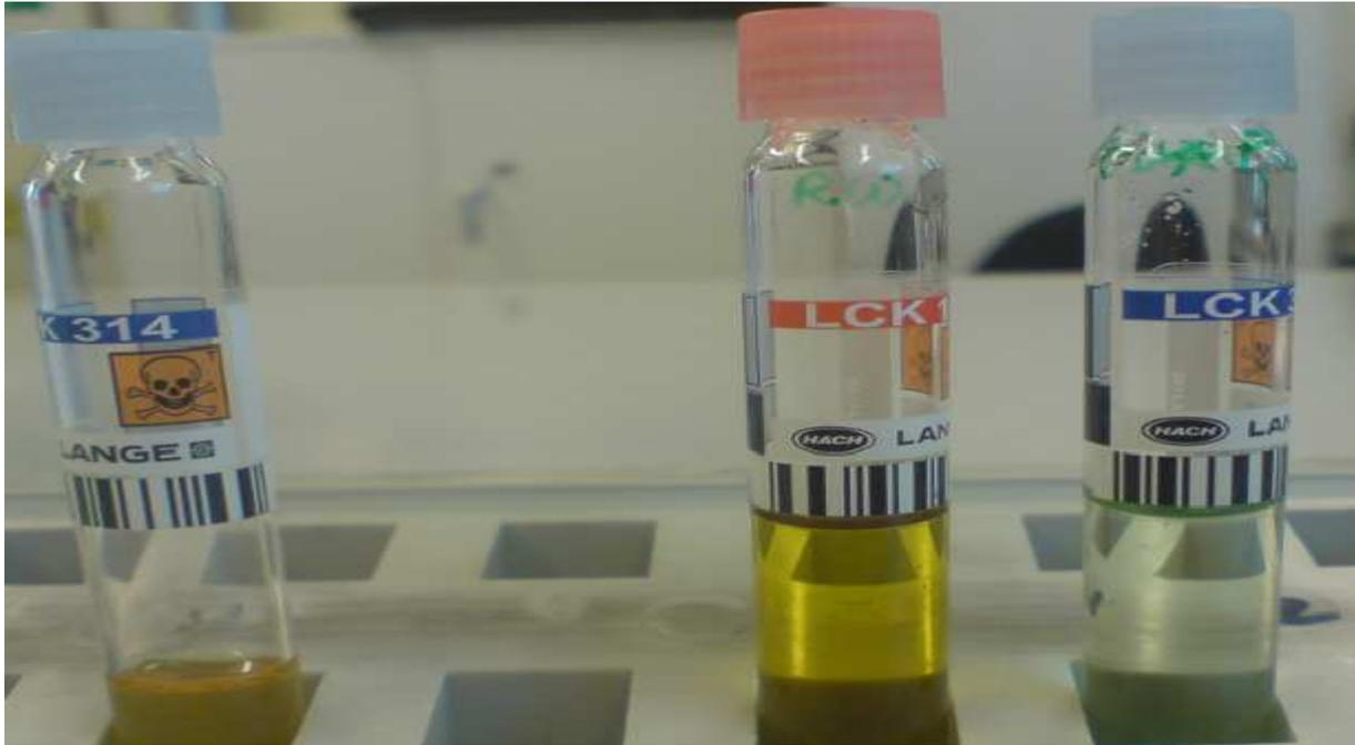
**Figure 6:** COD HACH-LANGE Cuvettes
