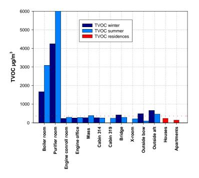
Figure 3. Concentration of TVOC in the various spaces onboard the icebreaker Oden. The information from Swedish residences is added for comparison. The dashed line represents the hygienically safe level of 300  $\mu$ g/m<sup>3</sup> as specified by the Federal Environment Agency of Germany (UBA).
