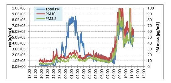
Figure 4. Particle concentration as a function of the operation mode of the main engines (ME): total number concentration (Total PN) and  $PM_{10}$  and  $PM_{2.5}$  mass concentrations as continuously measured by optical particle counter. 8 - 22 ME off, 22 - 03 ME on, 03 - 7:45 ME off 7:45 - 11:30 ME on.
