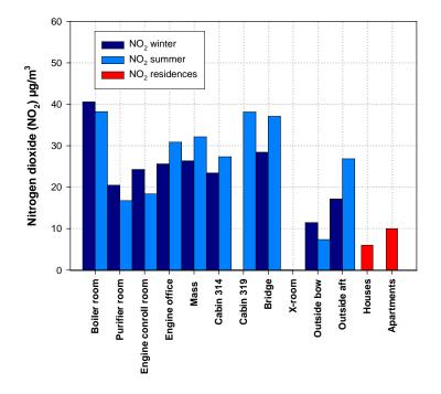
Figure 1. Concentration of  $NO_2$  in the various spaces onboard the icebreaker Oden. The information from Swedish residences is added for comparison.
