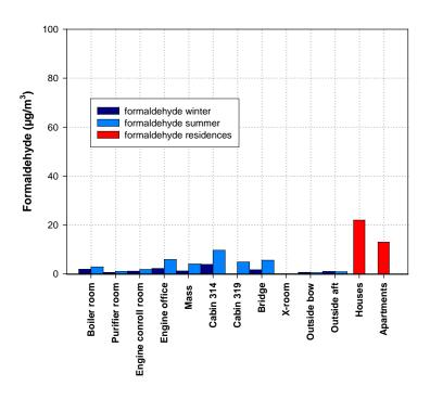
Figure 2. Concentration of formaldehyde in the various spaces onboard the icebreaker Oden. The information from Swedish residences is added for comparison.
