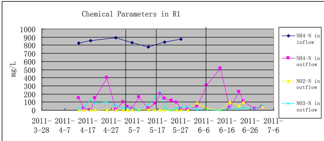
Fig. 15 The ammonium, nitrite and nitrate in R1.
