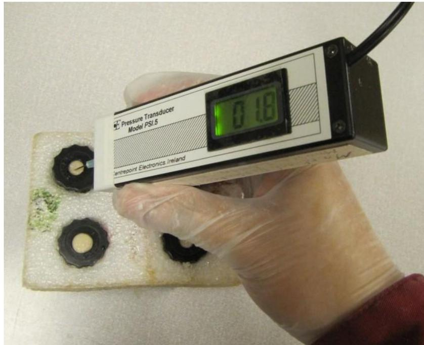
*Fig. 8 Measuring the pressure in SAA test.*
