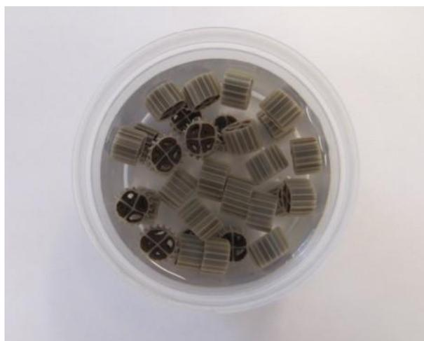
*Fig. 4 Biofilm used to build the reactor.*
